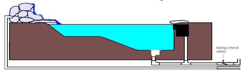
Swing check valve installed below water level in an easily accessed location will make keeping the pump and Turbovortex primed much more easy.
